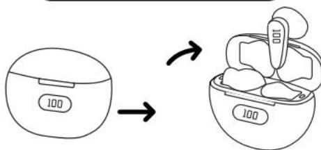
Open the charging compartment, the indicator lights of the headset flash alternately, and automatically pair with each other
