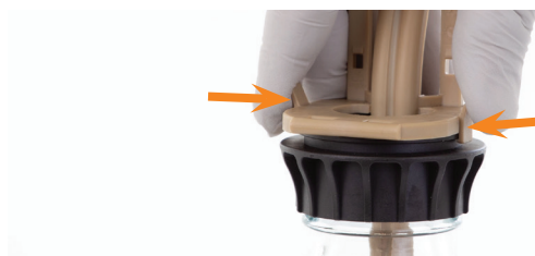
Figure 5. Attach the tube holder to the cap.
