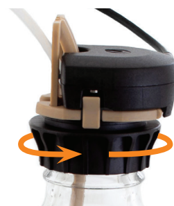
Figure 31. Remove the whole liquid level sensor assembly by unscrewing the cap. The cap rotates freely, independent of the attached tub holder and sensor.
