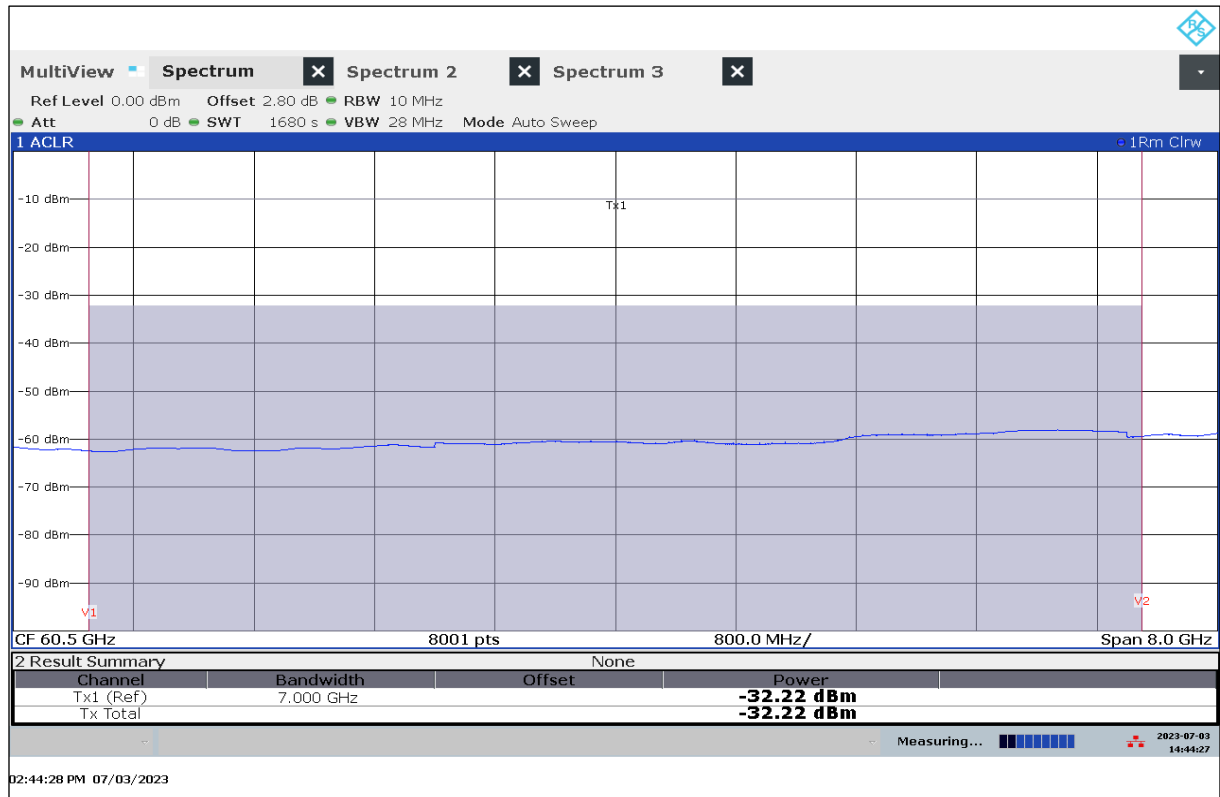
Plot 4: Channel Power within 57 GHz to 64 GHz
