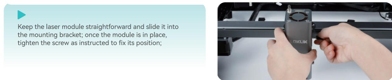
► Keep the laser module straightforward and slide it into the mounting bracket; once the module is in place, tighten the screw as instructed to fix its position;
