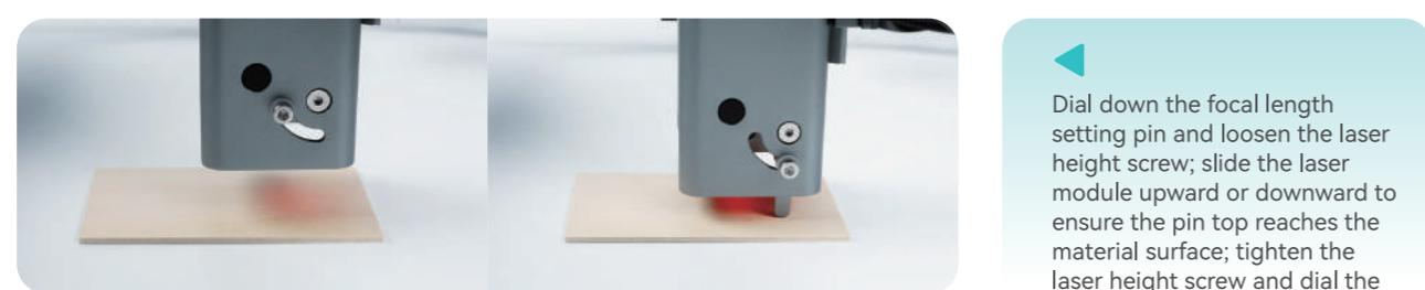
◀ Dial down the focal length setting pin and loosen the laser height screw; slide the laser module upward or downward to ensure the pin top reaches the material surface; tighten the laser height screw and dial the pin back to its original position;
