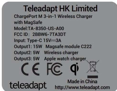
Specifications: Text is Black in color and justified. Labels are printed in indelible ink on permanent adhesive silk-screened onto the EUT or shall be affixed at a conspicuous location on the EUT.
