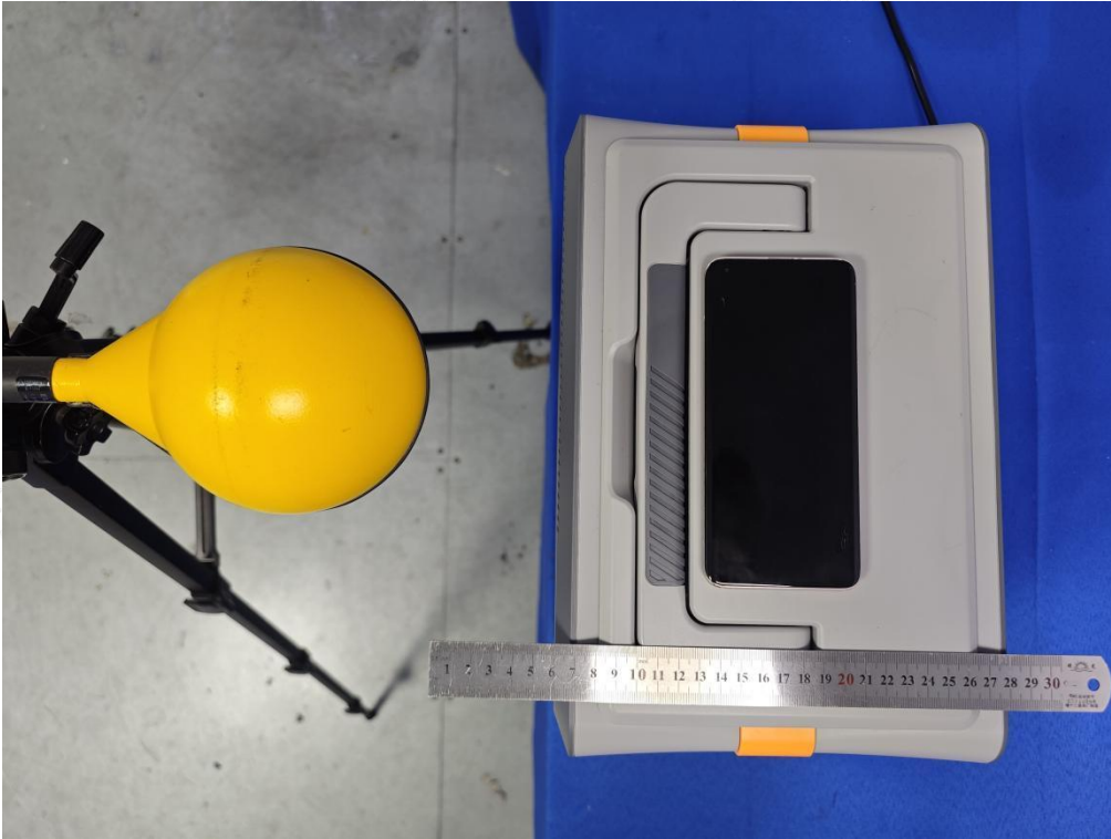
Test Position B(6cm) - Exposure photo from side edge surface-Rear(TM4)
