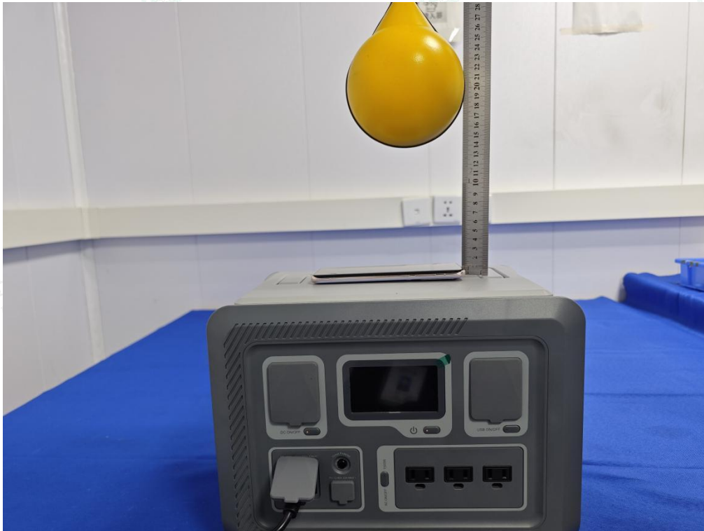
Test Position A (14cm) - Exposure photo from top surface (TM4)
