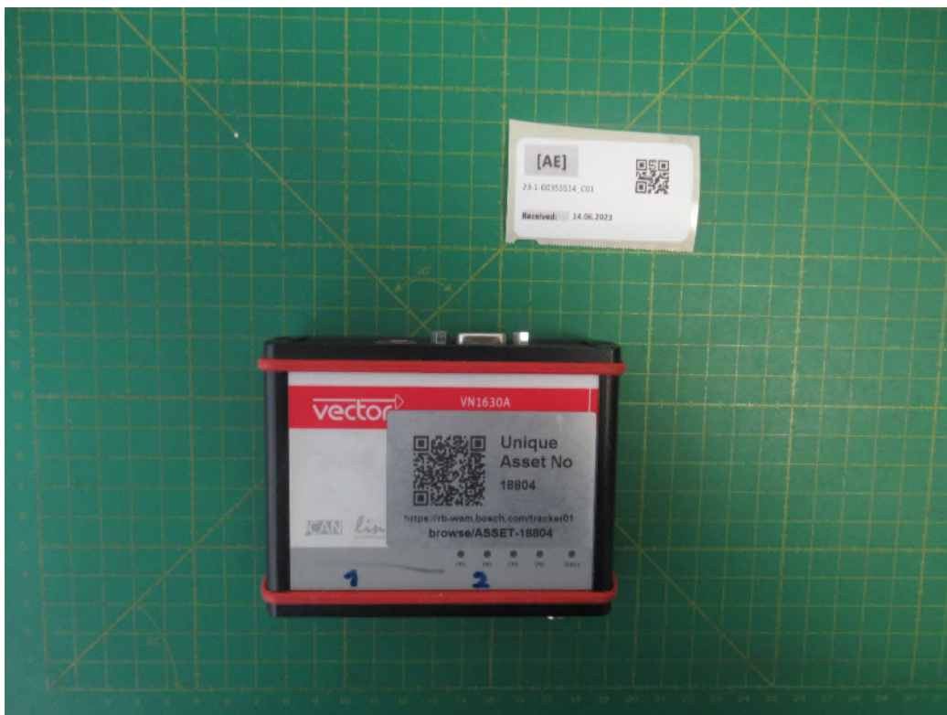
Fig. Ext.: 6 : Ext. - Front CAN/LIN Interface
