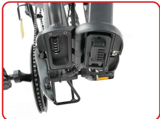
05. First, fold the frame and ensure that the front and rear frames are horizontally aligned. Next, push the folding handle towards the battery tube to ensure the folding handle is in the locked position.
