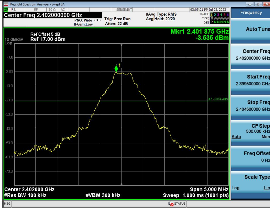
2 Spurious Emissions NVNT_ANT1_1-DH1_2402
