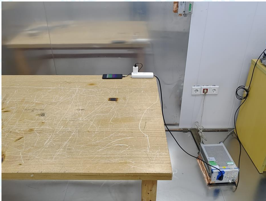
Photo of Setup for Conducted Emission
