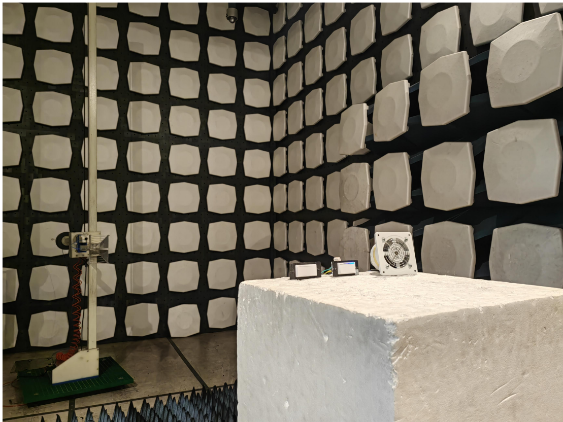
1 GHz to 40 GHz Radiated Spurious Emissions
