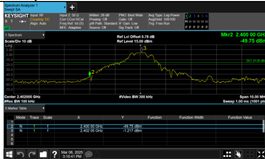
Out Of Band Emission GFSK_DH5_Channel 0
