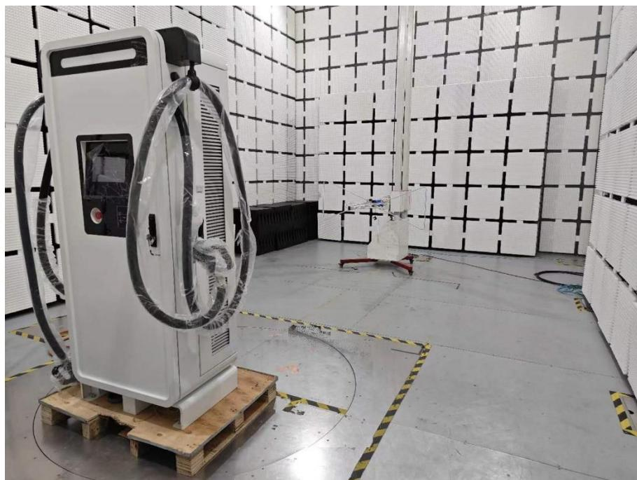
**Set-up for Conducted Emission**
