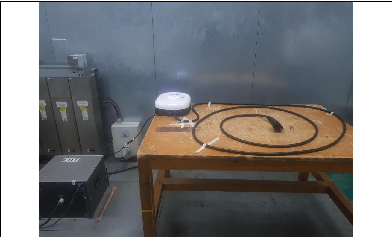
**- RADIATED EMISSION TEST****9 kHz ~ 30 MHz**
