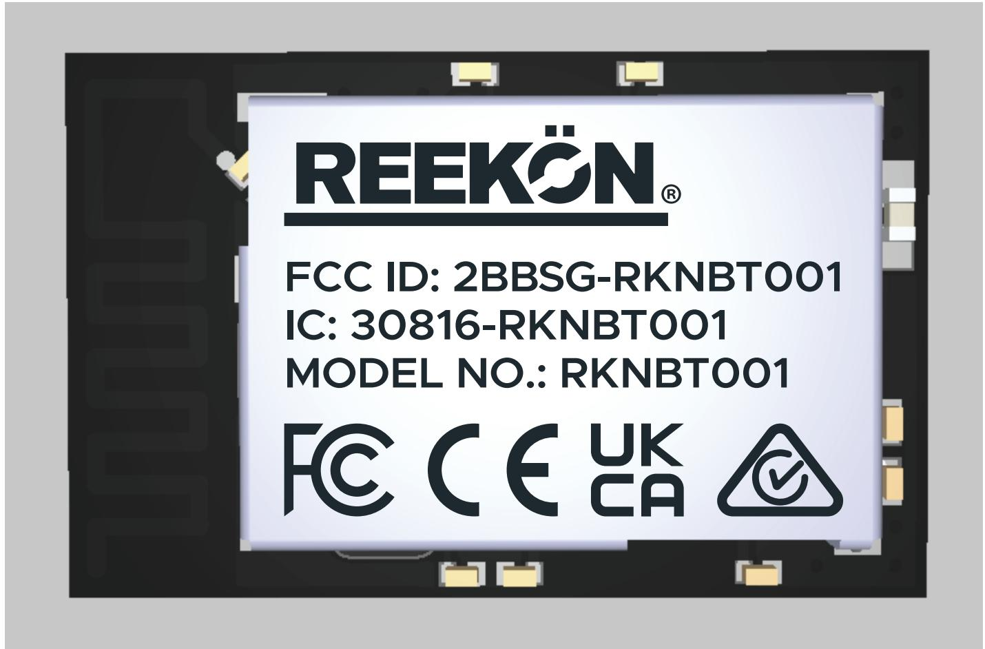
The labeling is laser etched into the RFI shield.
