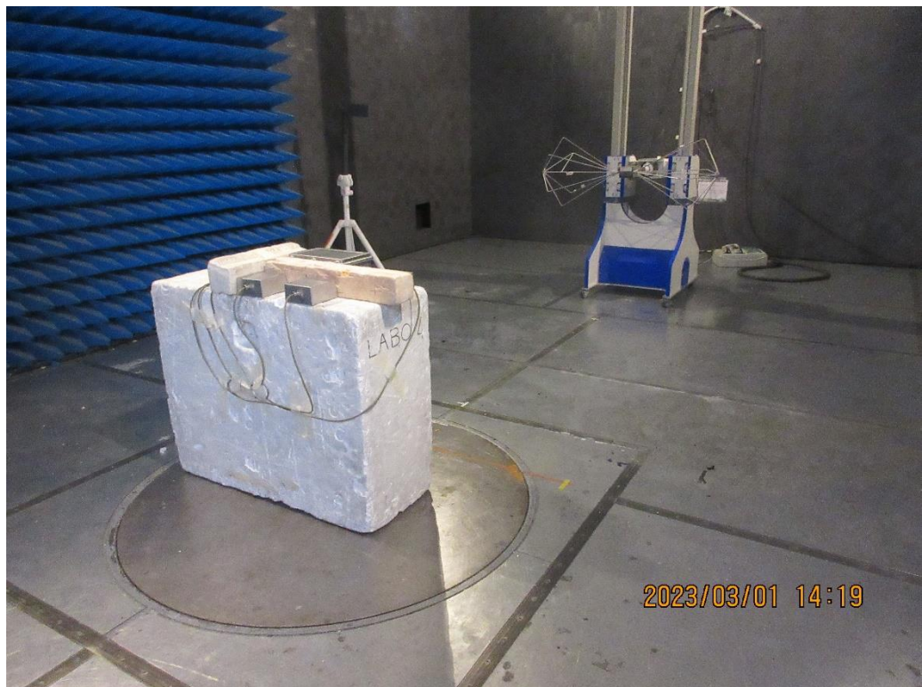
TEST SETUP PHOTOS – E.U.T. ON AZIMUTH 0° / FROM 30 MHz TO 200 MHz / HP
