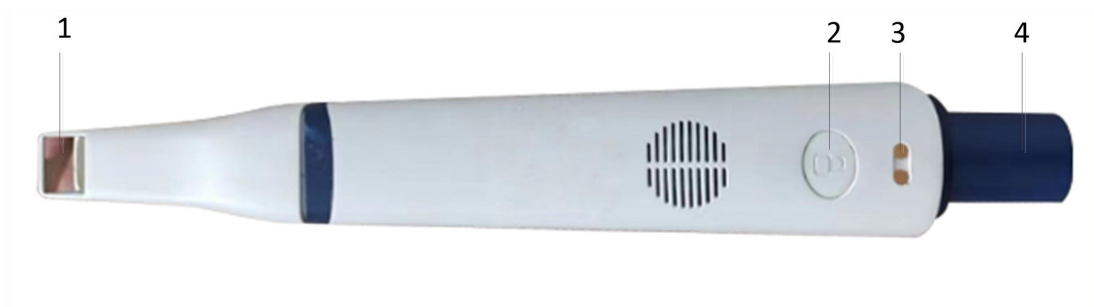
Fig. 1-2 Intraoral Camera (Camera of the Intraoral Scanner)
