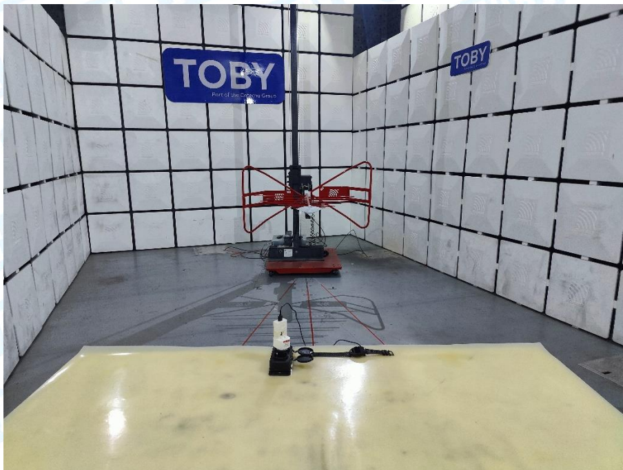
Photo of Setup for Radiated Emission (30MHz~1GHz)
