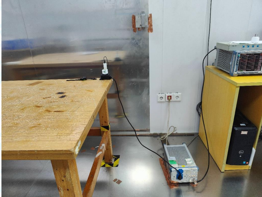
Photo of Setup for Radiated Emission (30MHz~1GHz)
