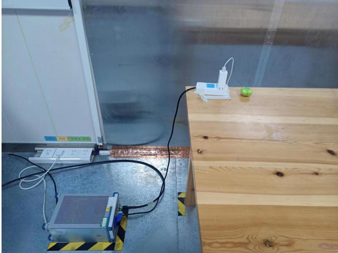
Conducted emission test setup
