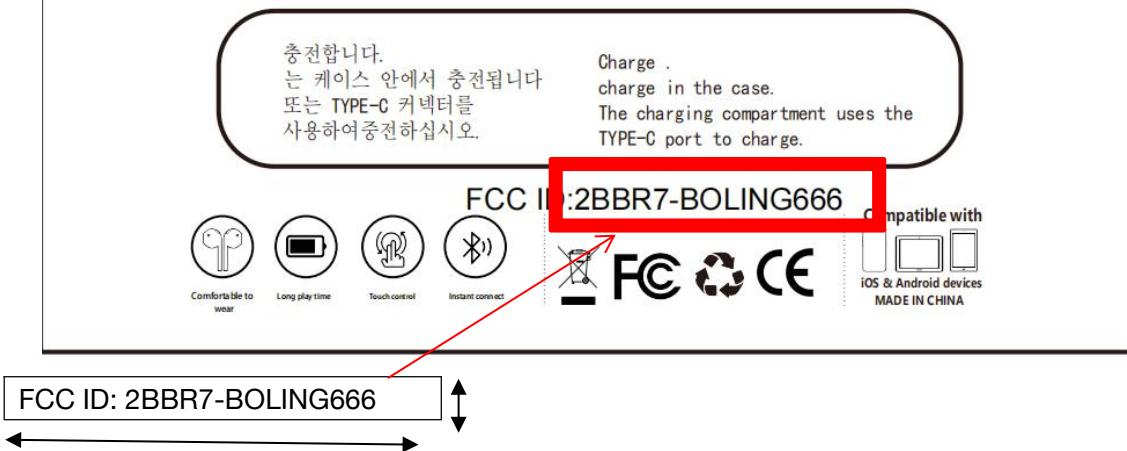
Note: Because EUT size is not suitable for printing FCC ID number label, FCC ID label is added on page 6 of the manual
