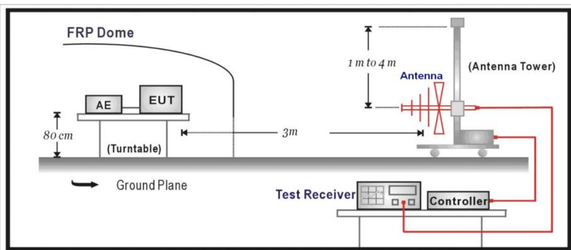
1GHz -40GHz Test Setup:
