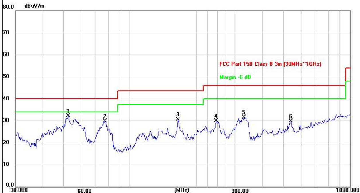
Antennal Polarity&amp; Test Distance: Vertical at 3m
