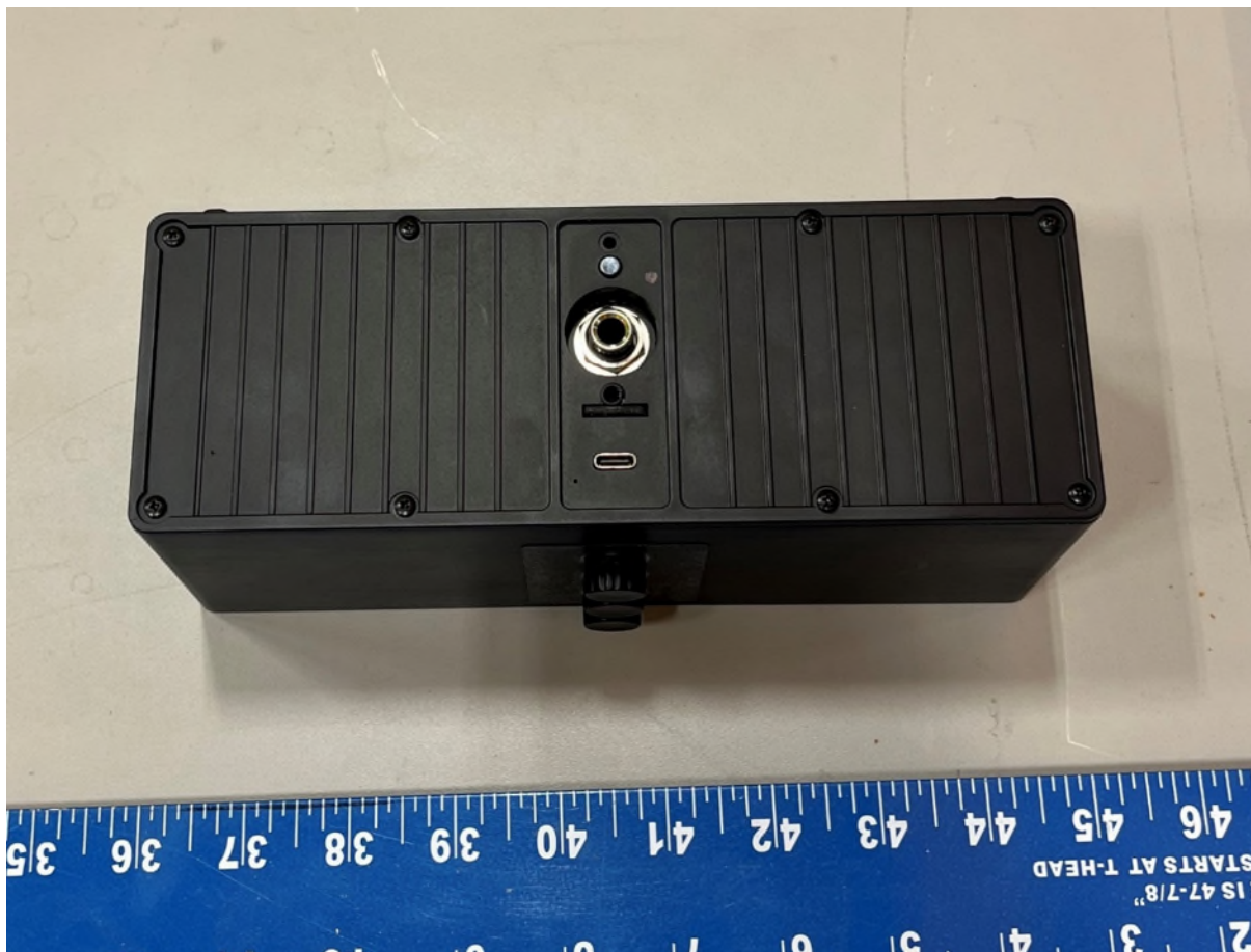
Figure 3 – Back view with I/O ports
