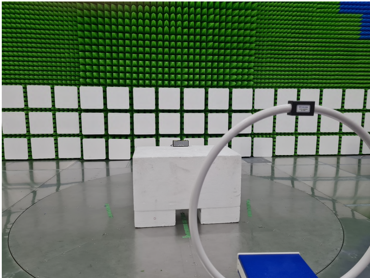
Figure 4 – Radiated Emissions Setup 9kHz – 30MHz
