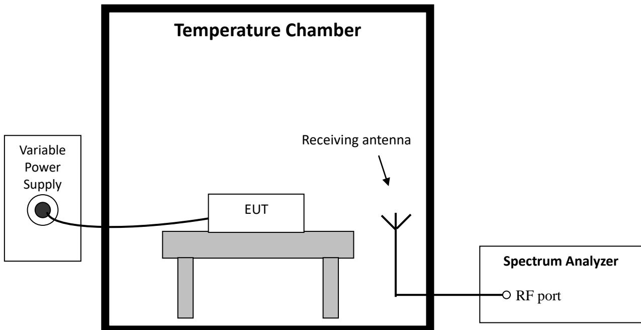
**6.3 Test procedure and test setup**
