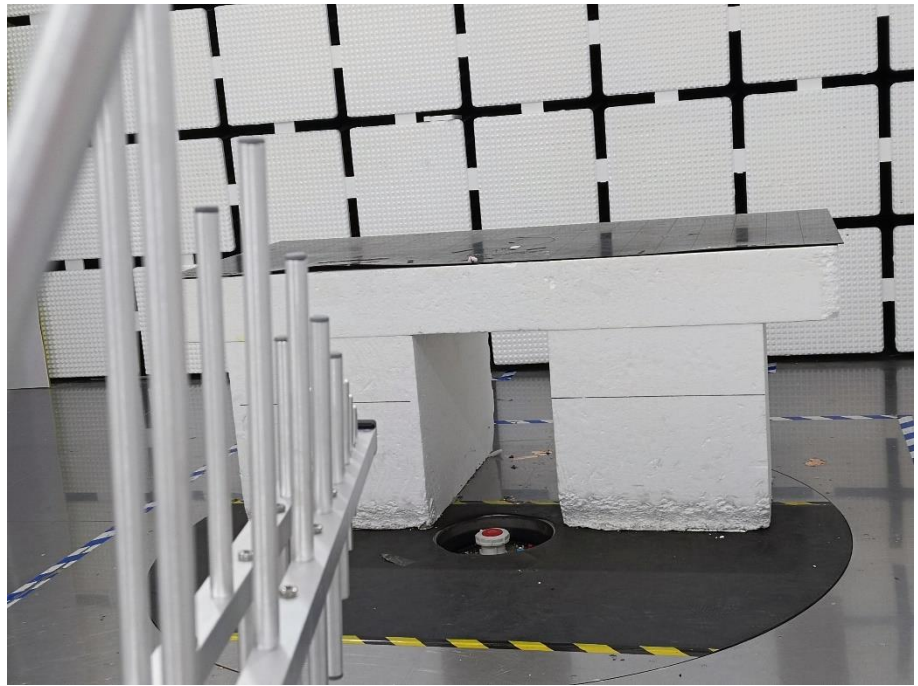
Radiation Emission Test Setup (30MHz to 1GHz)
