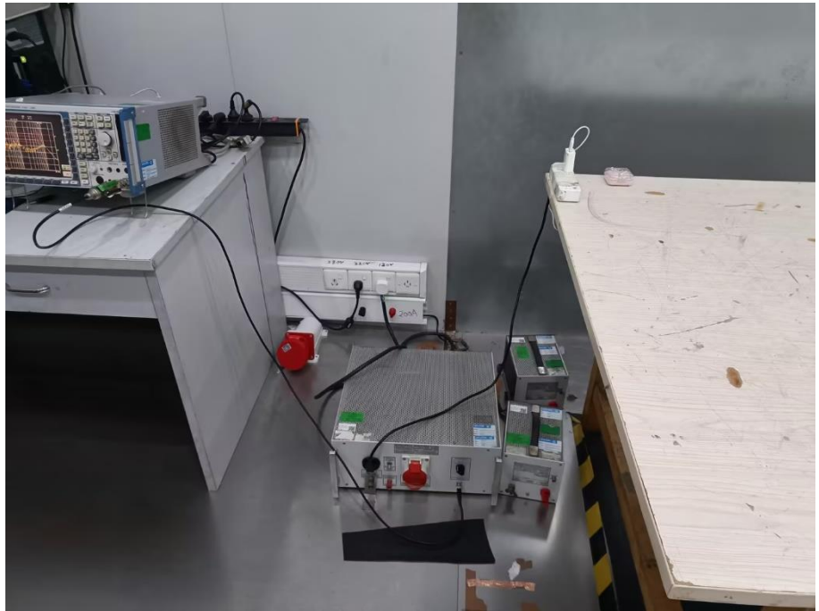
Conducted Emission Test Setup
