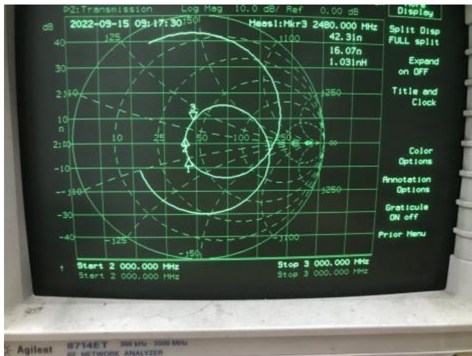
Figure 3 keyboard Antenna S11
