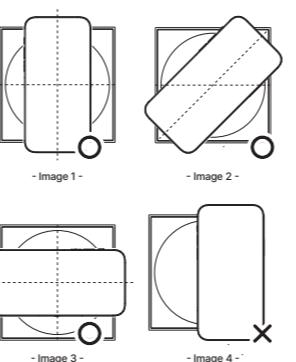
Please place the product and the device as shown in Images 1, 2, and 3, ensuring they are aligned at the center. If the device is placed incompletely as shown in Image 4, the charging efficiency may be reduced.
