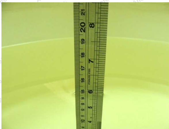
Photo of Liquid Height for Body SAR
