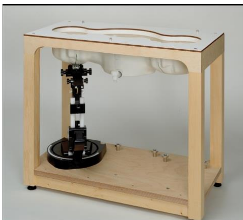
Picture C.11: SAM Twin Phantom
