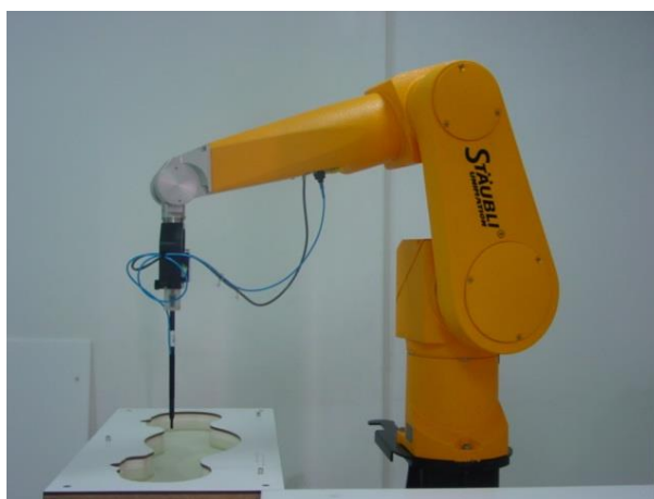
Picture D.6 Specific Absorption Rate Test Layout
