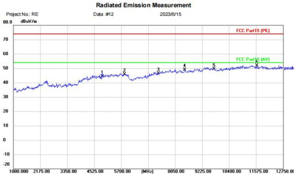
Site: Limit: FCC Part15 (PK) Polarization: **Vertical** Temperature: (C)
