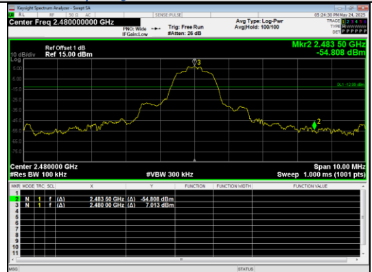
Out Of Band Emission \pi/4 DQPSK_2-DH5_Channel 78
