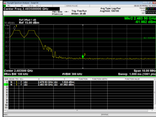
Out Of Band Emission(Right) GFSK_DH5_Channel Hopping
