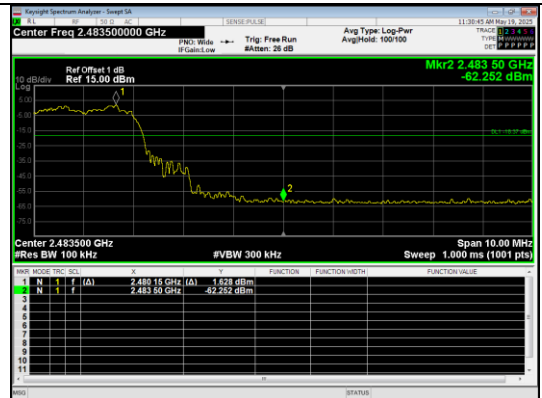
Out Of Band Emission(Right) 8DPSK_3-DH5_Channel Hopping
