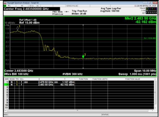
Out Of Band Emission(Right) \pi/4 DQPSK_2-DH5_Channel Hopping
