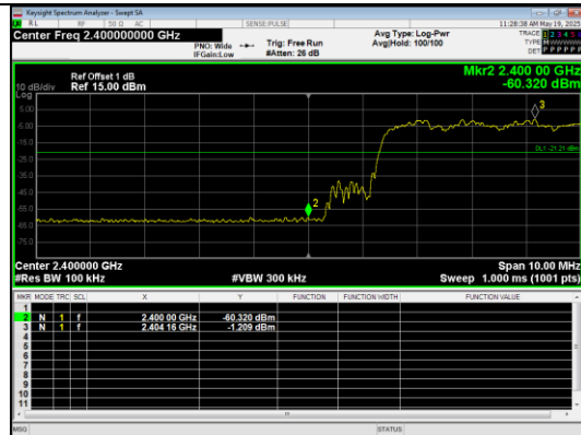
Out Of Band Emission(Left) 8DPSK_3-DH5_Channel Hopping
