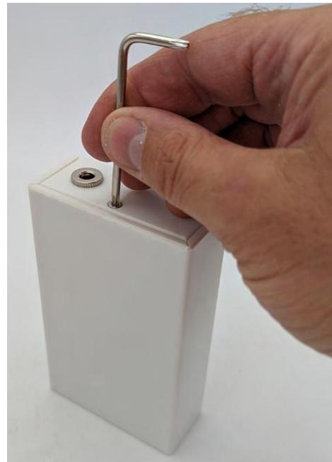
**3. Using the included security wrench, remove the T10 screw from the underside of the white enclosure.** The cover unclips from the top side by slightly pushing out the cover sides so that it can slide off.
