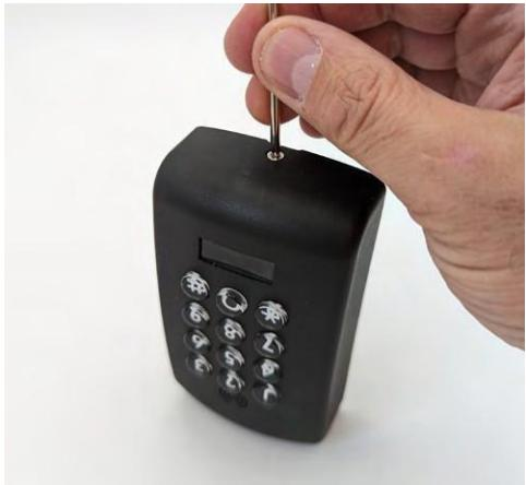
7. Remove the T10 security screw from the keypad using the included wrench.
