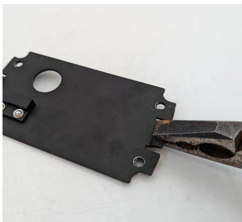
**11. If fitting the gasket, use pliers to carefully bend the top tap up slightly.** This makes aligning the keypad easier. There is no need to do this if fitting the rainshield.
