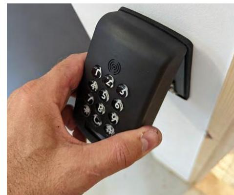
**14. Hold the keypad at an angle and insert into the backplate.** It must be perfectly aligned. If it will not locate, try bending the tab a 'little' more, but not too much as it could snap.
