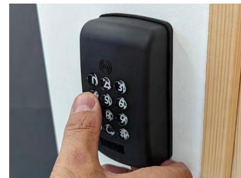
Enter the PIN code from the previous step. The keypad should beep twice and you should hear the strike release.
