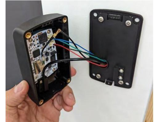
**13. Feed the 4 cables through the hole, making sure to pull them through the hole in the enclosure.** Do not pull tight, you should leave some slack cable within the keypad body.
