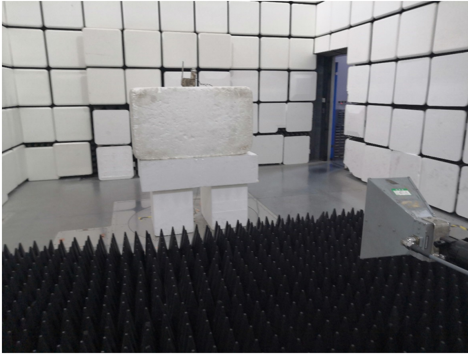
Picture 1 Radiated Spurious Emissions Test setup
