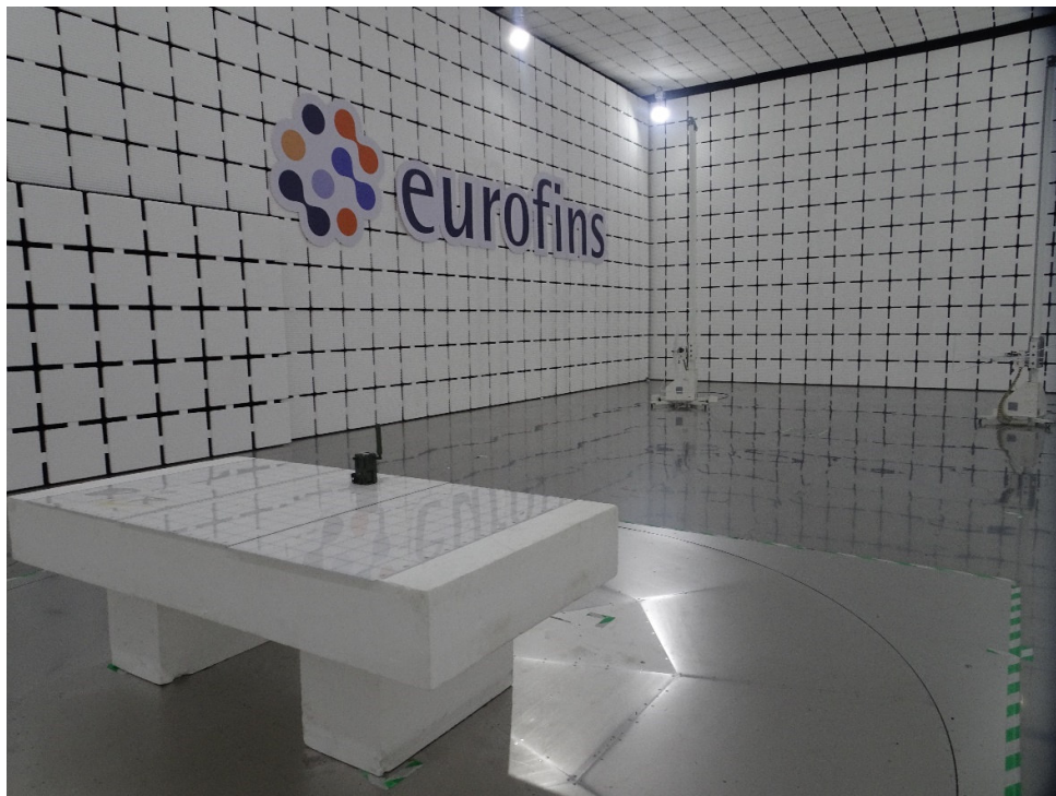
Picture 1: Radiated Emission Test Setup
