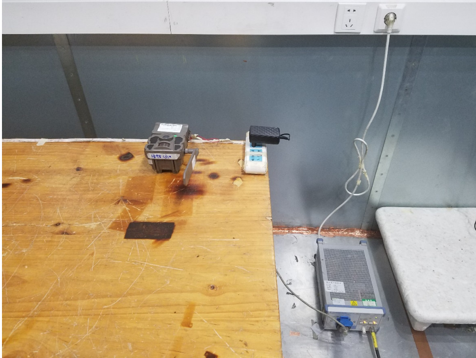
Picture 2: Conducted Emissions Test Setup
