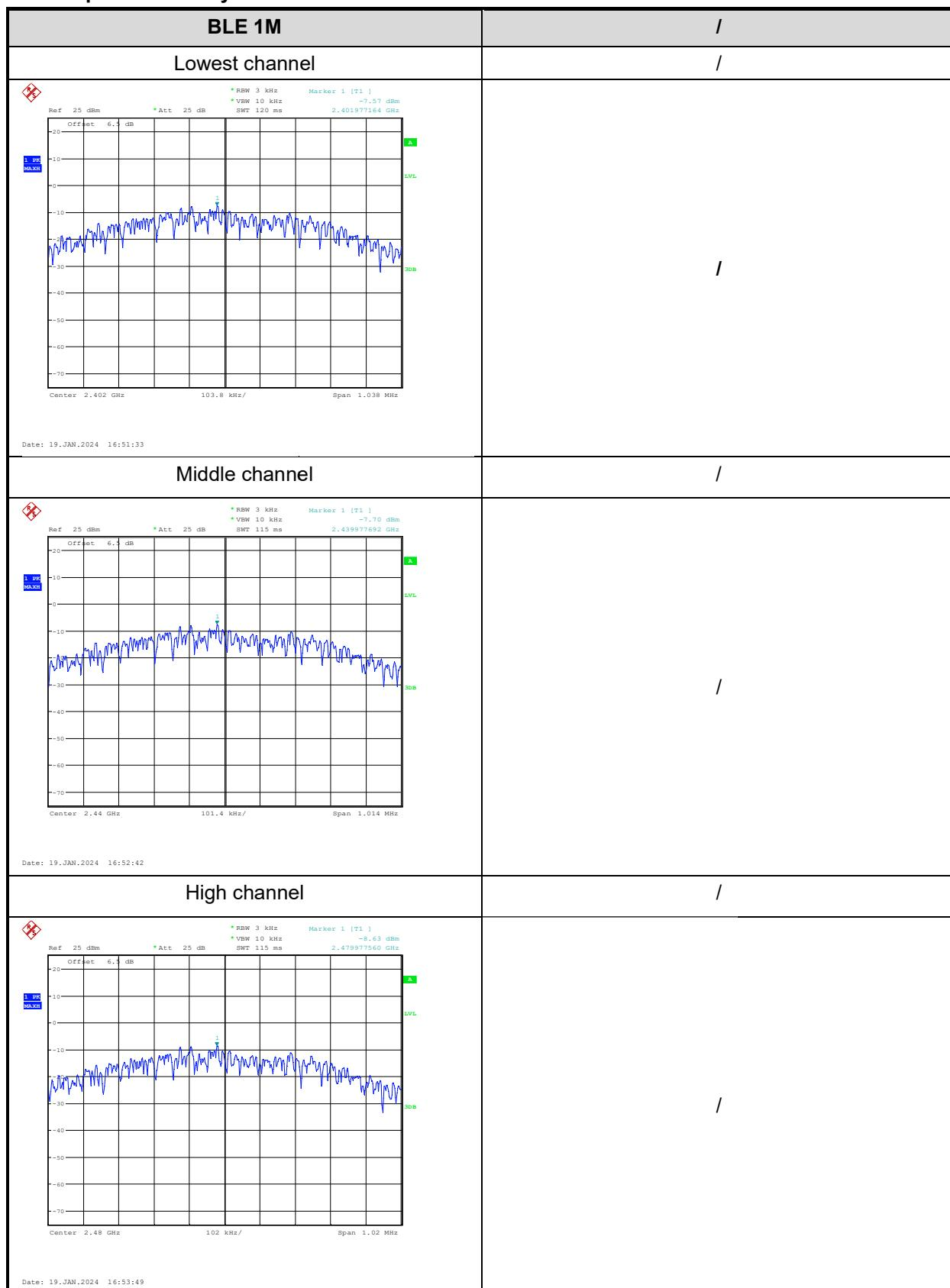
100kHz Bandwidth of Frequency Band Edge:
