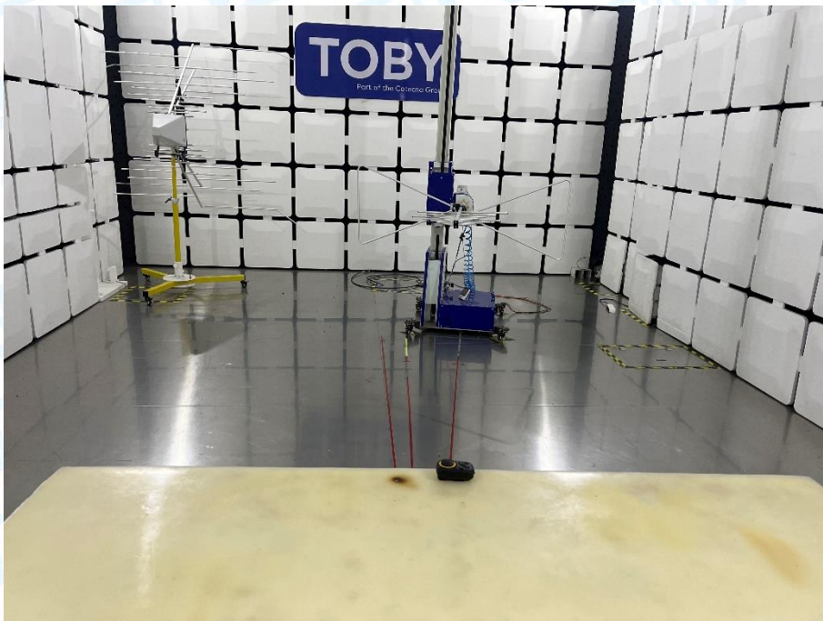
Photo of Setup for Radiated Emission (30MHz~1GHz)
