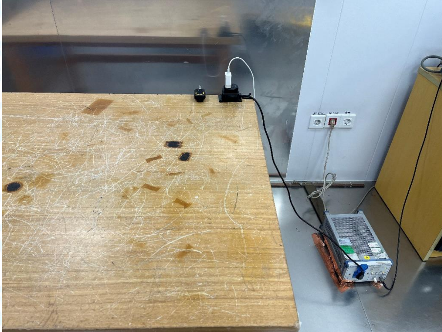
Photo of Setup for Radiated Emission (30MHz~1GHz)
