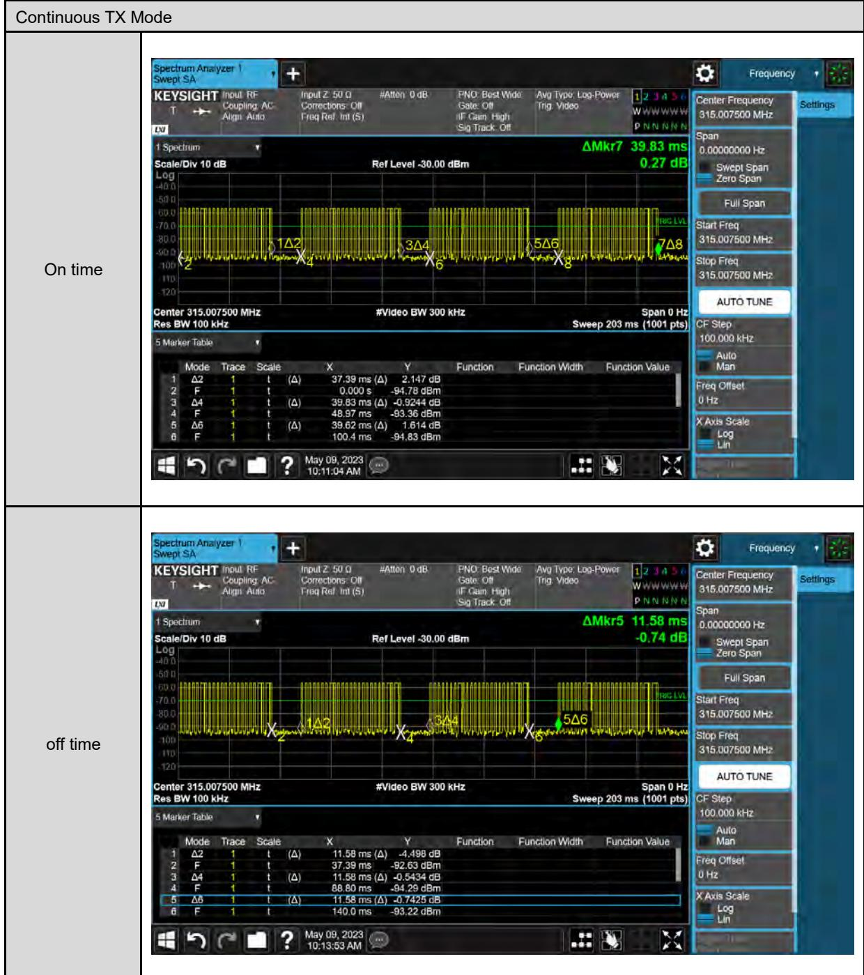
The EUT was complied with the requirement of FCC 15.231 (a) (1), which employed a switch that will automatically deactivate the transmitter within less than 5 seconds of being released.
