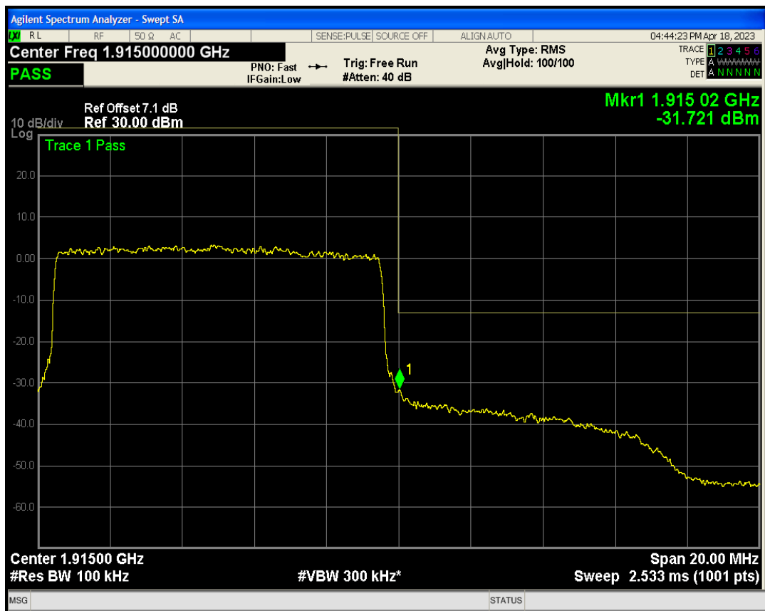
Band25 QPSK BW=15MHz Channel=26115 RB Size=75 Position=#0
