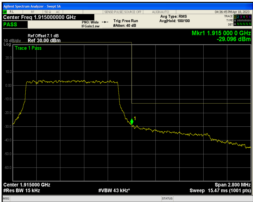
Band25 QPSK BW=3MHz Channel=26055 RB Size=15 Position=#0
