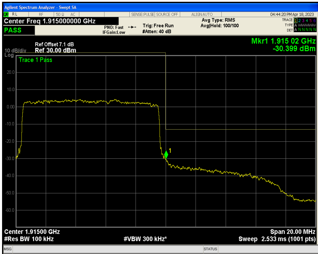
Band25 QAM16 BW=10MHz Channel=26640 RB Size=50 Position=#0
