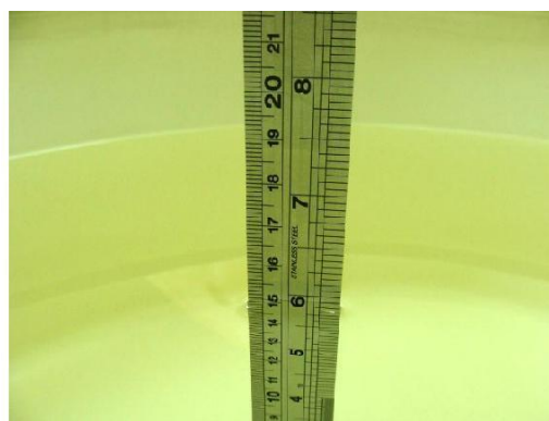
Fig 7.2 Photo of Liquid Height for Body SAR
