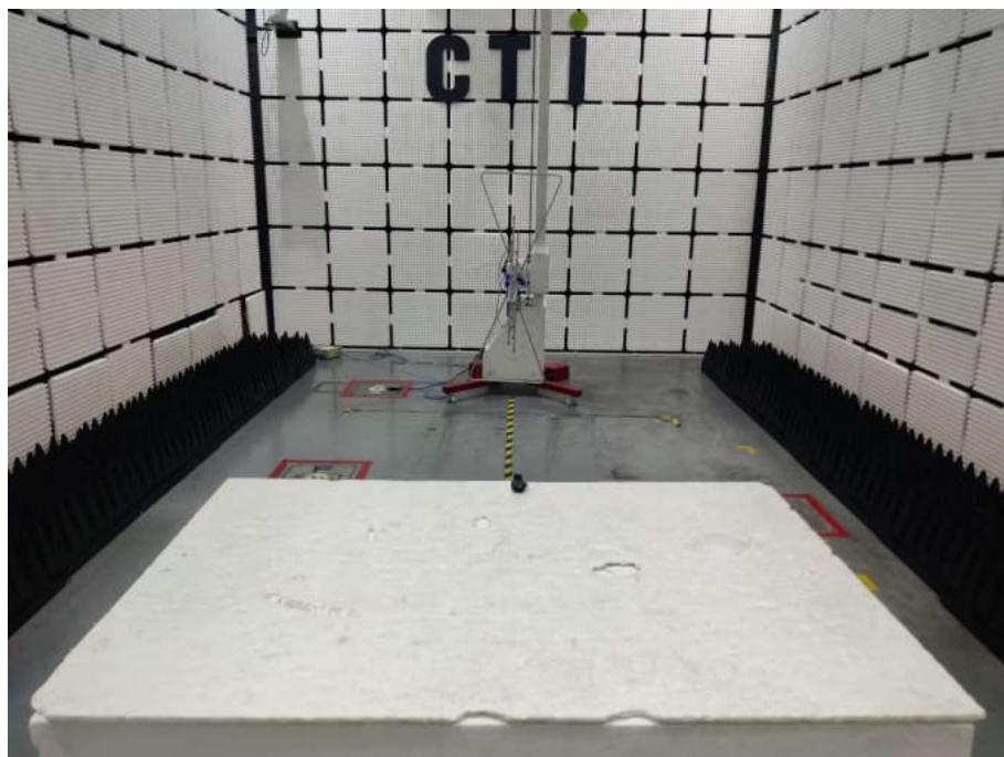
Radiated spurious emission Test Setup-1(Below 1GHz)
