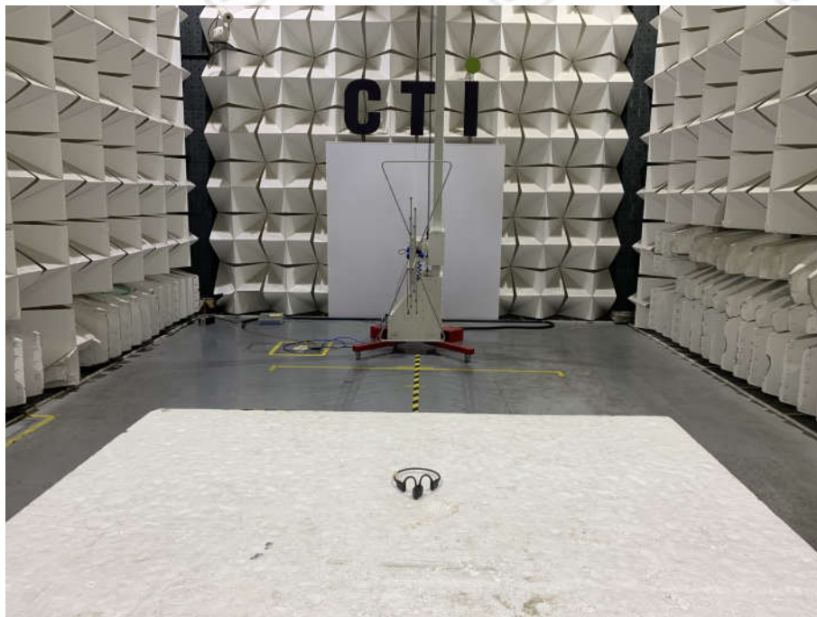
Radiated spurious emission Test Setup-1 (Below 1GHz)
