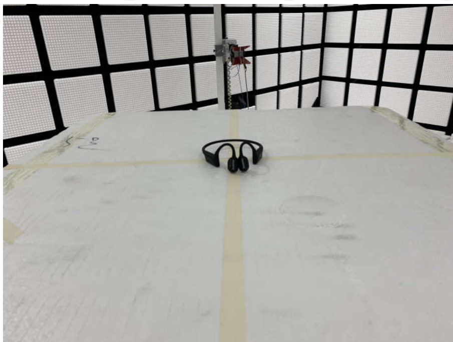
Radiated spurious emission Test Setup-2 (Above 1GHz)
