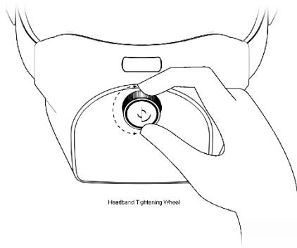
1. After placing the Lynx-R1 on your head, adjust the headband tightness by turning the adjustment wheel at the back of the device.
