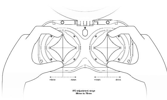
2. Move the lenses left and right manually to adjust the device to your inter-pupillary distance ; making sure they are place properly in front your eyes.
