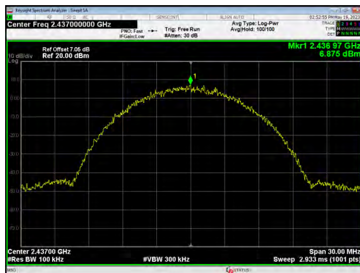
Tx. Spurious NVNT b 2437MHz Ant1 Ref
