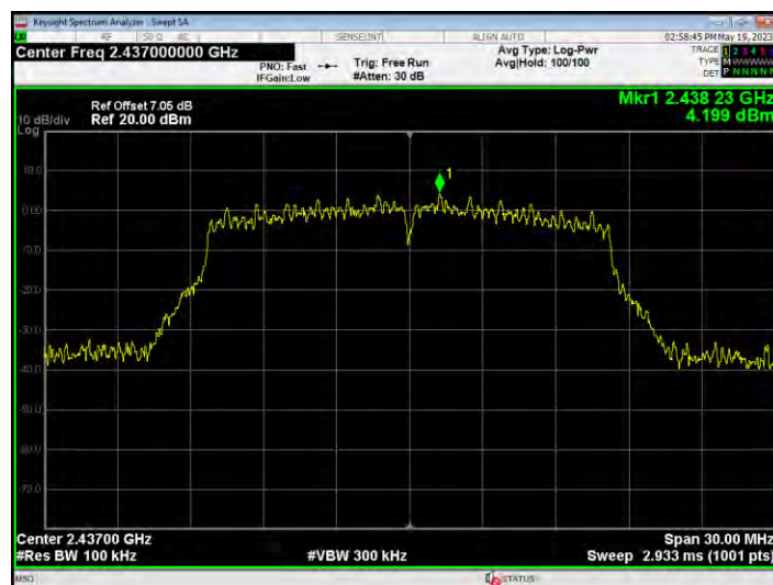
Tx. Spurious NVNT g 2437MHz Ant1 Ref
