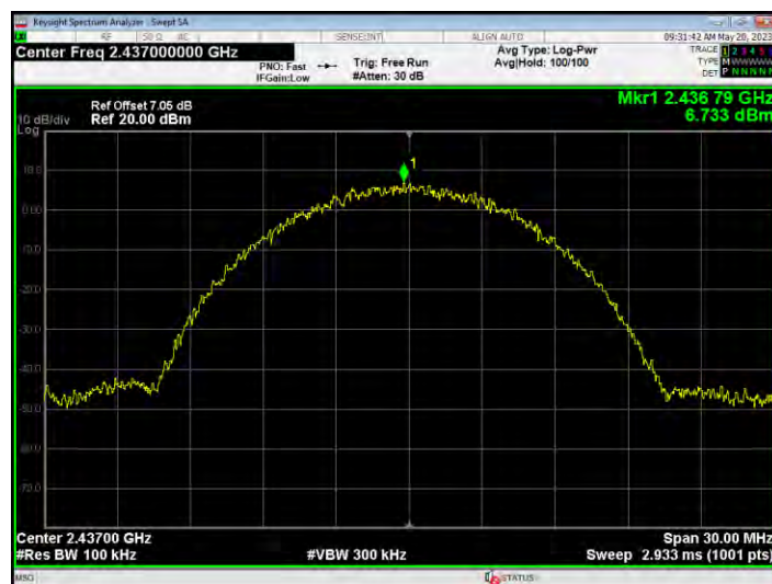
Tx. Spurious NVNT b 2437MHz Ant1 Ref
