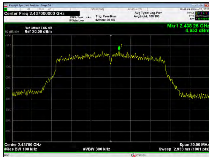
Tx. Spurious NVNT g 2437MHz Ant1 Ref
