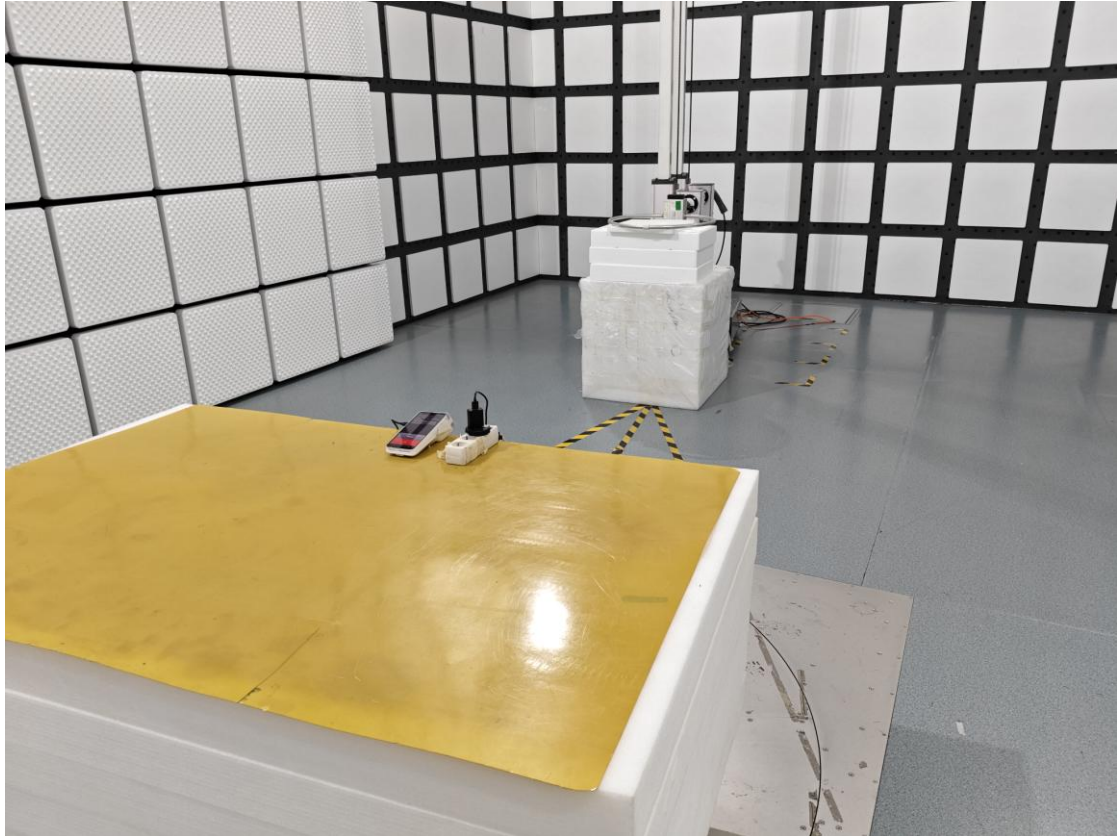
Radiated Spurious Emissions Test View (9kHz-30MHz) (Test Mode 1)
