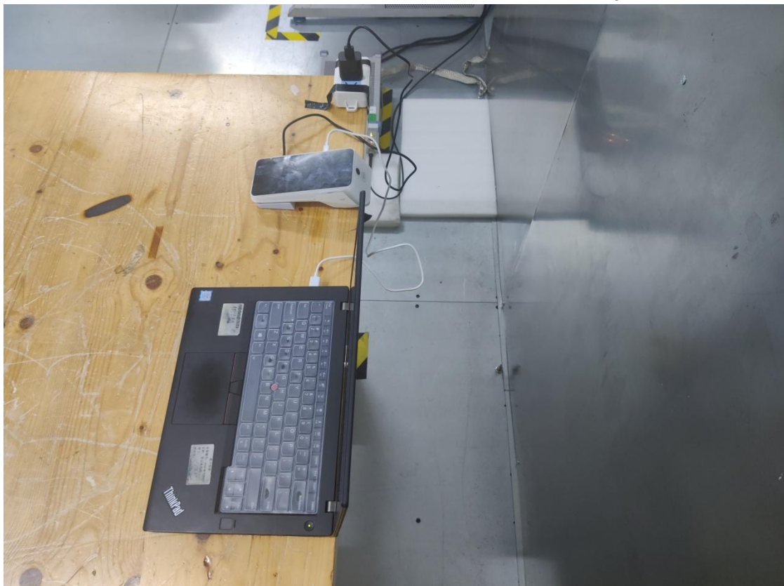
Photo of Power Line Conducted Emission Measurement-Side View(Test Mode 3&4)
