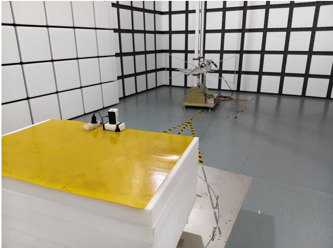
Radiated Spurious Emissions Test View (30MHz-1GHz) (Test Mode 1&2)
