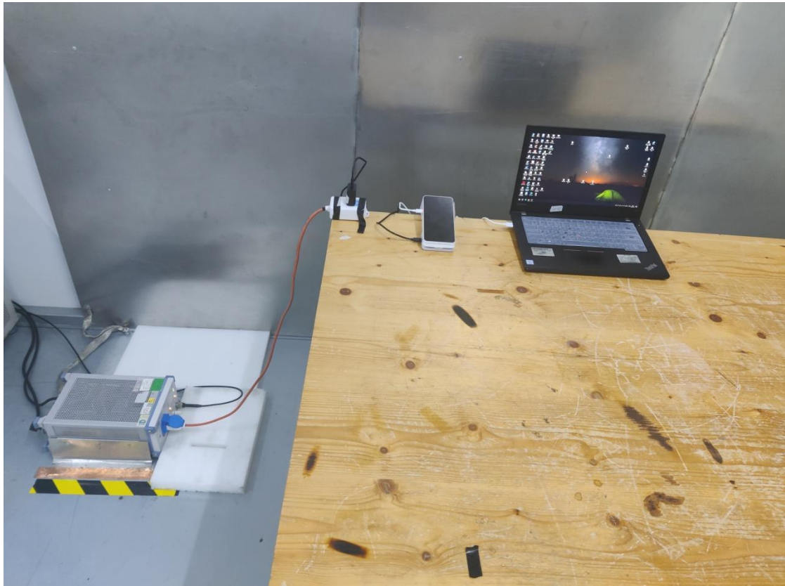
Photo of Power Line Conducted Emission Measurement-Front View(Test Mode 3&4)
