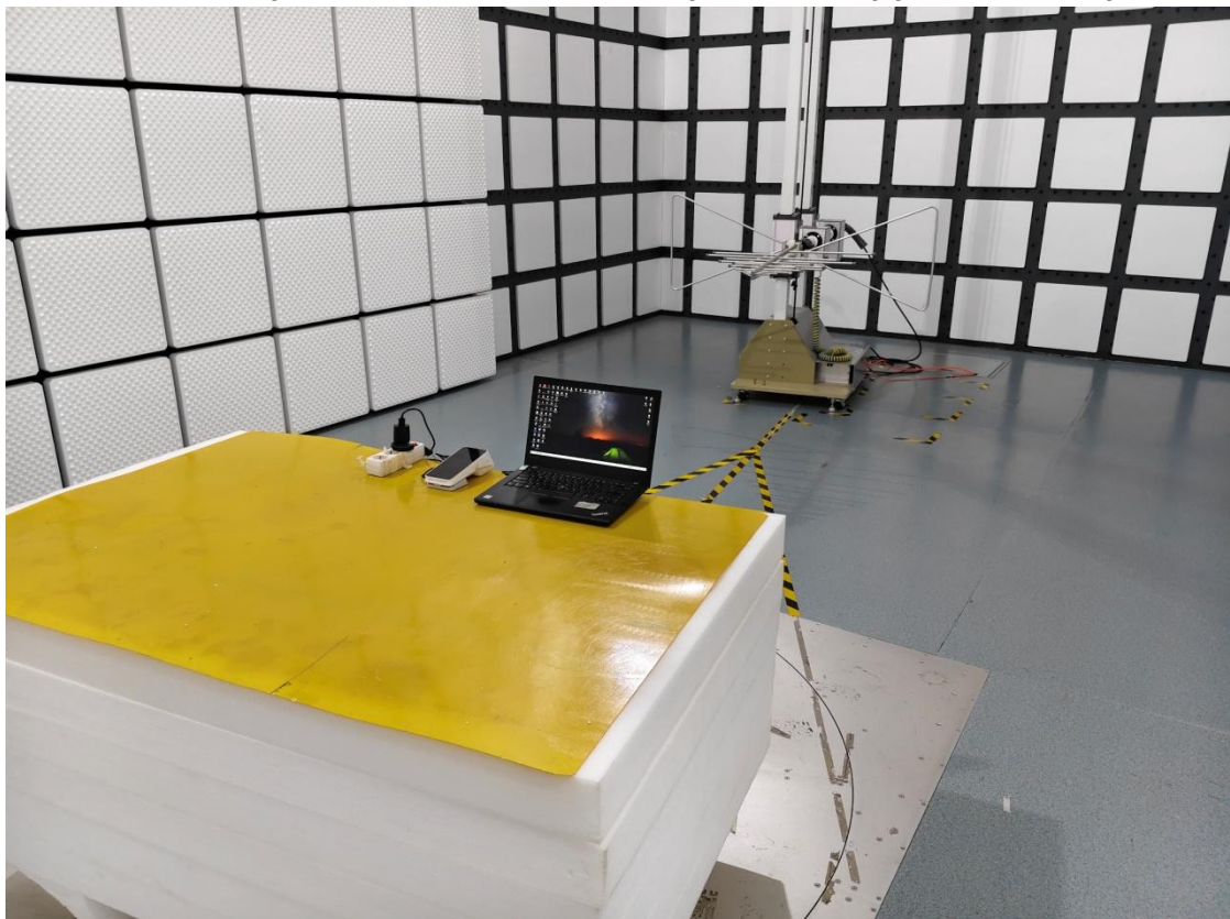
Radiated Spurious Emissions Test View (30MHz-1GHz) (Test Mode 3&4)
